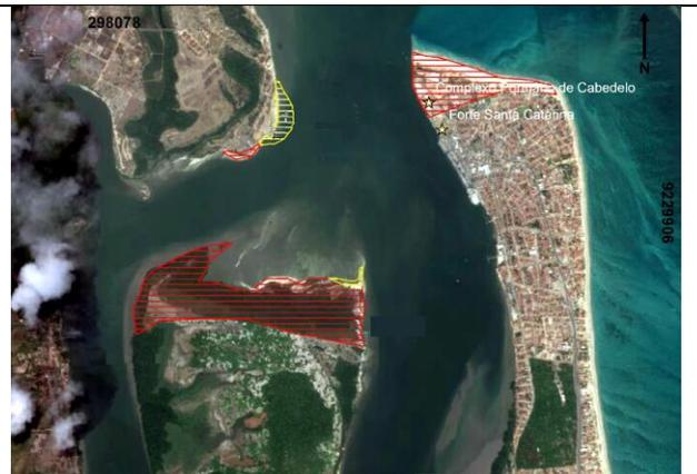
F) The dashed areas were those have changed, in red are those of progradation and, in yellow, sectors in process of erosion. *Source: adapted from Google(2015).*
