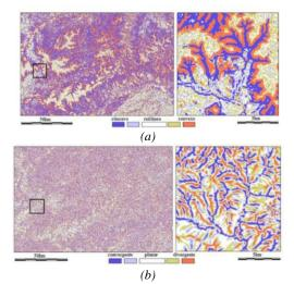
Figure 3- (a) Vertical curvature in five classes. (b) - Horizontal curvature in three classes. Source: Valeriano (2008).
