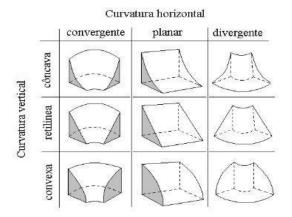
Figure 4- Terrain shapes: Combination of curvatures to characterize terrain shapes. Source: Valeriano (2008).
