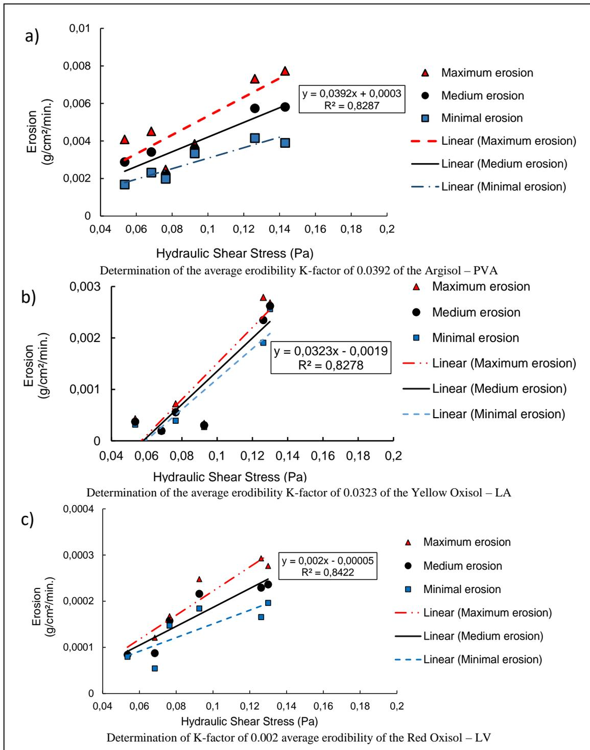
Figure 10 - Determination of the average erodibility K-factor of the samples. Source: The authors.
