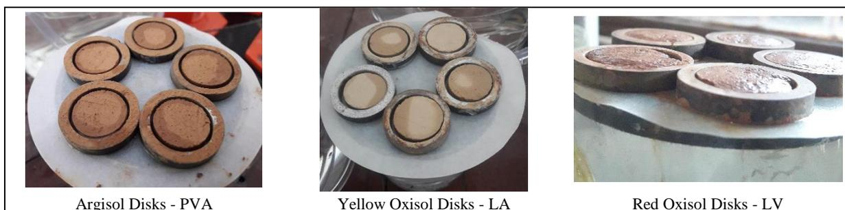
Figure 8 - Water reabsorption procedure in the disks used. Source: The authors.
