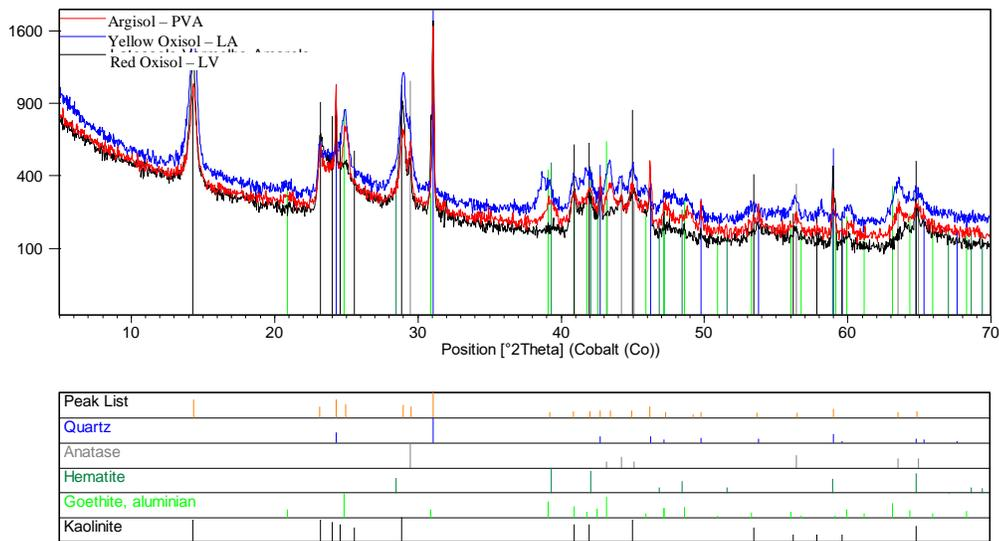
Figure 6 Mineralogical identification by X-ray diffraction. Source: The authors.
