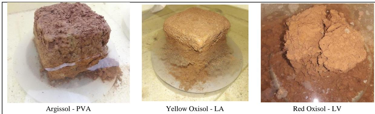
Figure 9 - Slaking test with partial immersion.. Source: Os authors.
