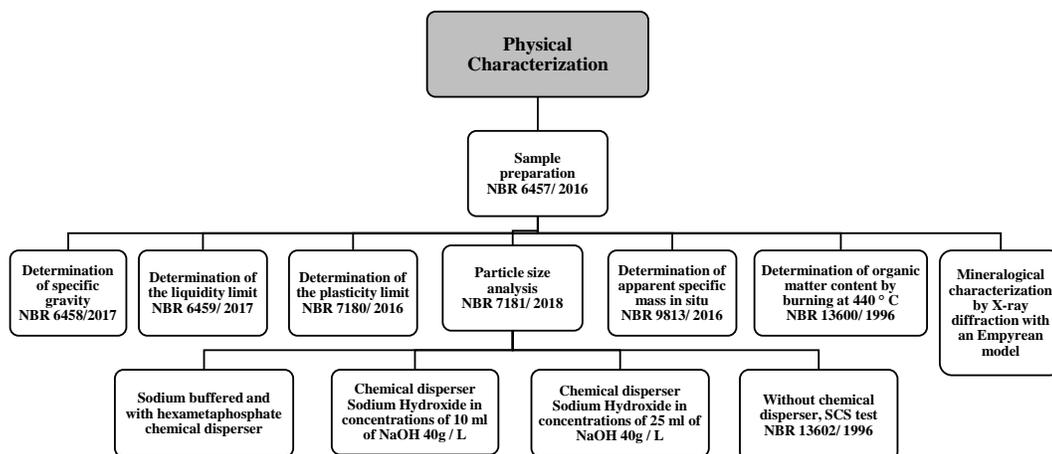
Figure 4 - Flowchart of sample characterization tests. Source: The authors.
