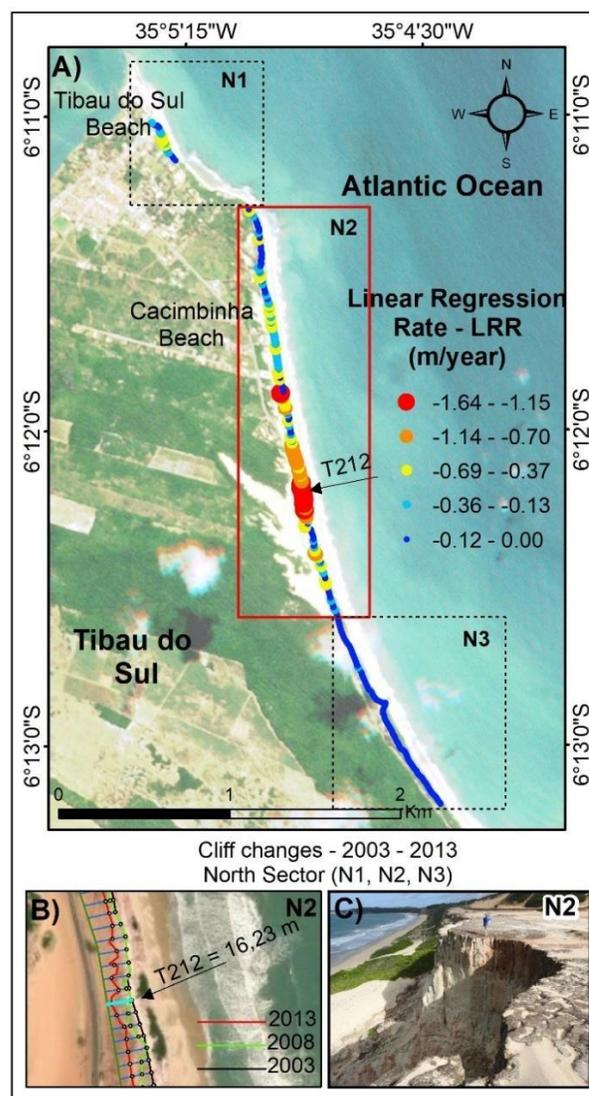
Figure 7 – Changes in the cliff retreat rate in the North sector: (A) Map representing the linear regression rate (m/year) between 2003 and 2013 identifying the most critical subsector (N2); (B) Transect T21, with maximum retreat and near the access road; (C) panoramic view of transect T212.
