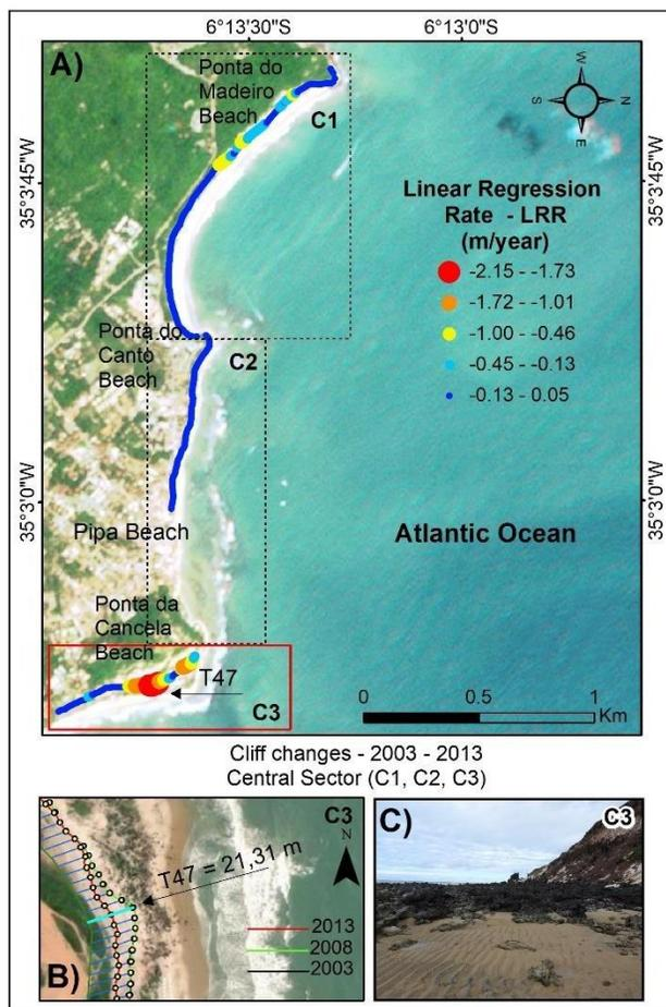
Figure 8 - Changes in the cliff retreat rate in the Central sector: (A) Map representing the linear regression rate (m/year) between 2003 and 2013, identifying the most critical subsector (C3); (B) Transect T47 with maximum retreat; (C) Panoramic view of transect T47.
