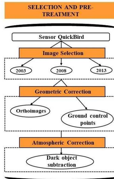
Figure 4 – Flowchart of the first stage: selection and procedures involved in the pre-processing of high-resolution multispectral images from the QUICKBIRD satellite.
