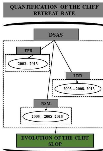
Figure 6 – Flowchart of the third stage: DSAS statistics module used to quantify the cliffline retreat rates.
