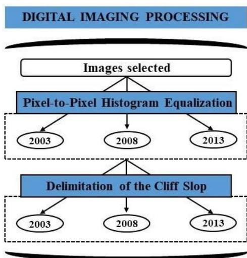
Figure 5 – Flowchart of the second stage: main DIP treatments to enhance and delimit the cliff edges.
