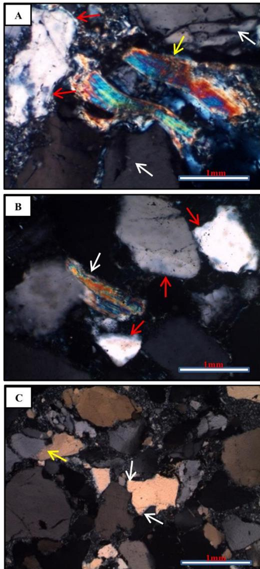
Figura 11 - Diagenetic Products: A) Muscovite folded between quartz grains (yellow arrow), fractured quartz grains (white arrows), with dissolution and secondary growth (red arrows) (PX); B) Secondary growth of quartz (red arrows) and inter-grain muscovite (white arrow) (PX); and C) Prismatic quartz projections (white arrows), and sutured contact between quartz grains (yellow arrow) (PX).
