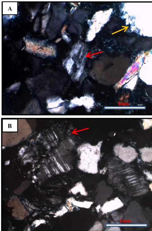
Figura 8 - Dissolved and fractured primary constituents: A) orthoclase and quartz grain undergoing dissolution (red and yellow arrows, respectively, XP); B) Fractured plagioclase grain (arrow, XP).
