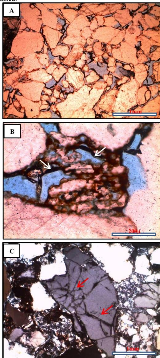
Figura 7 - Types of porosity: A) Intergranular primary porosity (blue; PP); B) Secondary porosity by partial dissolution of feldspar (arrows; PP); and C) Secondary porosity by the fracturing of a quartz grain (arrows, XP).
