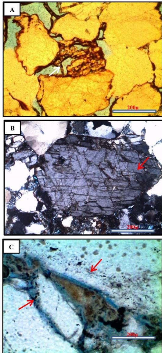
Figura 12 - Diagenetic products: A) partially dissolved feldspar generating secondary porosity (arrow, PP); B) Fracture of feldspar generating secondary porosity (arrow, PX); and C) Clay shrinkage (arrows) generating secondary porosity (PP).
