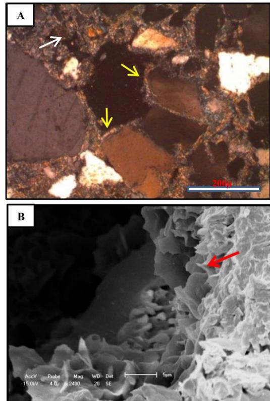
Figura 9 - Infiltrated clay: smectite/illite cuticle recovering grains (yellow arrows) and as microcrystalline aggregate (white arrow) (XP); and B) SEM image showing smectite recovering a grain (arrow), with evidence of illitization.
