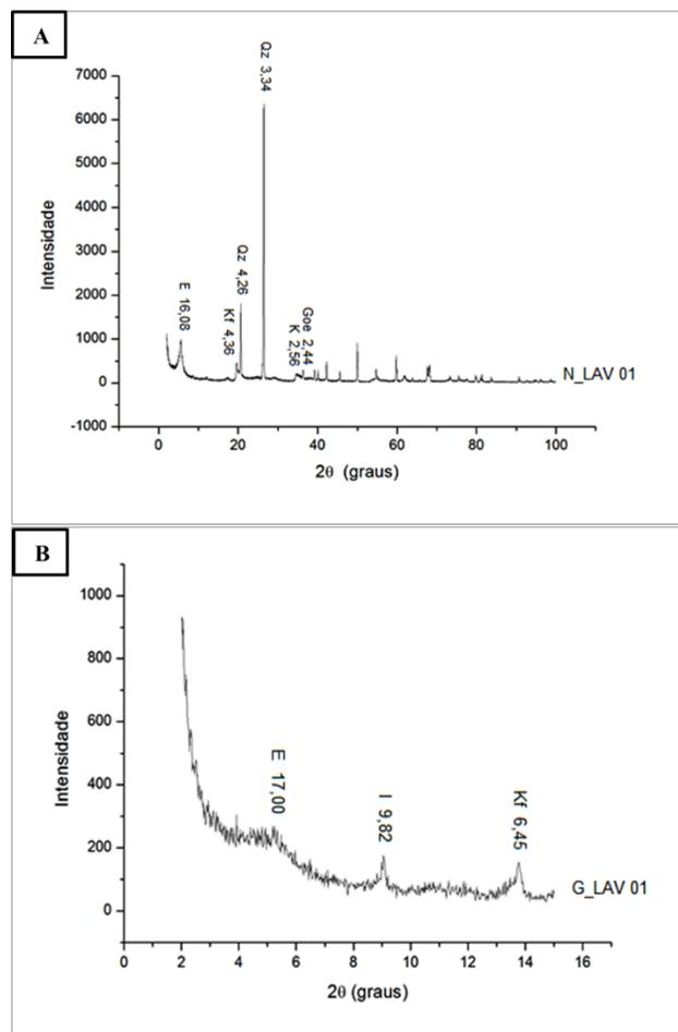
Figura 10 - Clay minerals: A) XRD without treatment (*in natura*); B) XRD with glycosylation treatment. **Legend:** Qz – quartz; Kf – feldspar; E – smectite; I – illite; K – kaolinite; Goe – goethite.
