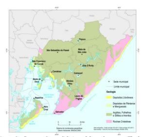
Figure 6 - Degree of consolidation of the vadose zone. The least consolidated materials are found in coastal deposits, mangroves and sedimentary rocks. Crystalline rocks have a higher degree of consolidation. Source: Authors (2019).
