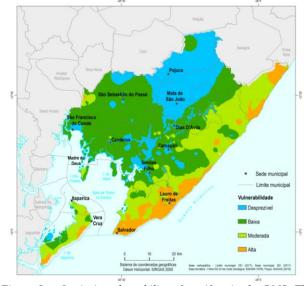
Figure 8 - Intrinsic vulnerability of aquifers in the RMS. The areas most vulnerable to contamination are coastal areas, whose material is predominantly sandy, the amount of rain is greater, the static level is less and the aquifer is free. Source: Source: Authors (2019).
