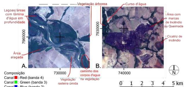
Figure 5 – R(4)G(3)B(2) composite (true color). All bands derive from the Sentinel-2 MSI VIS.
