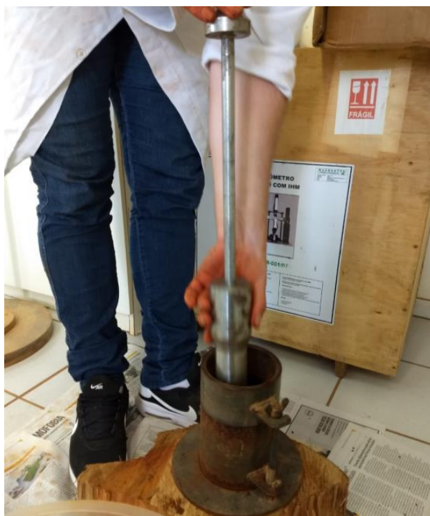
Figure 3 – Soil compaction using Proctor. Source: Author (2019).
