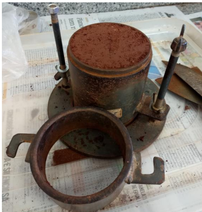
Figure 4 – Cylinder with compacted soil to collect density data. Source: Author (2019).
