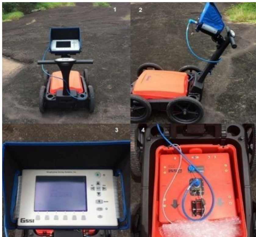
Figure 3 - GPR GSSI3000 with the 270MHz antenna, 1) Complete equipment, operator view; 2) Equipment in profile; 3) Control unit; 4) 270 MHz antenna.
