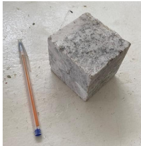
Figure 5 – Detail of cubic specimens, measuring 7 cm of edges to carry out the test resistance to uniaxial compression of rocks
