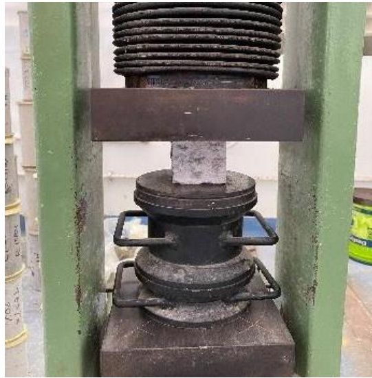
Figure 3 – Hydraulic press used to determine the uniaxial compressive strength Source: Authors (2021).
