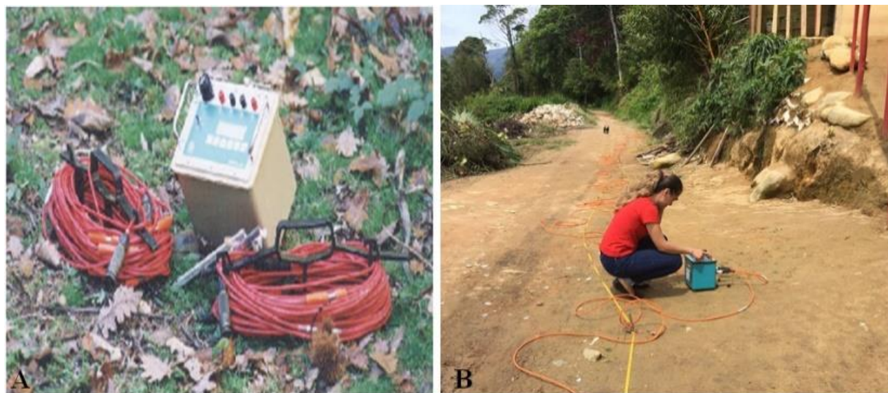
Figure 7 - (A) Syscal kid Switch-24 Equipment. Source: Authors (2022).
