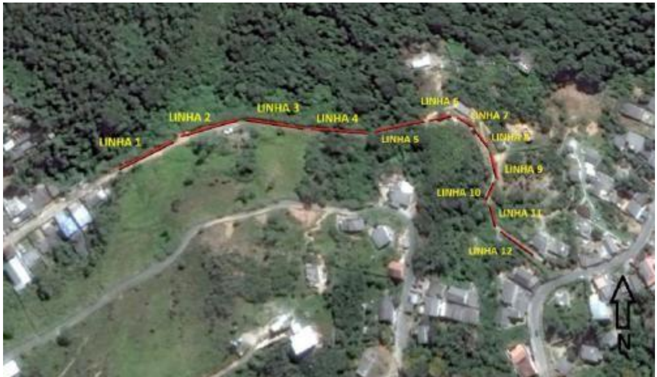
Figure 2 - GPR acquisition lines at Mato Grosso Street. Source: Marques (2016).
