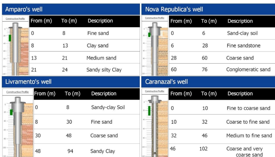
Figure 4 – Geological profiles of the 04 wells, close to the study area, used for analysis of the local geology. The green demarcations determine the dynamic level oscillation.
