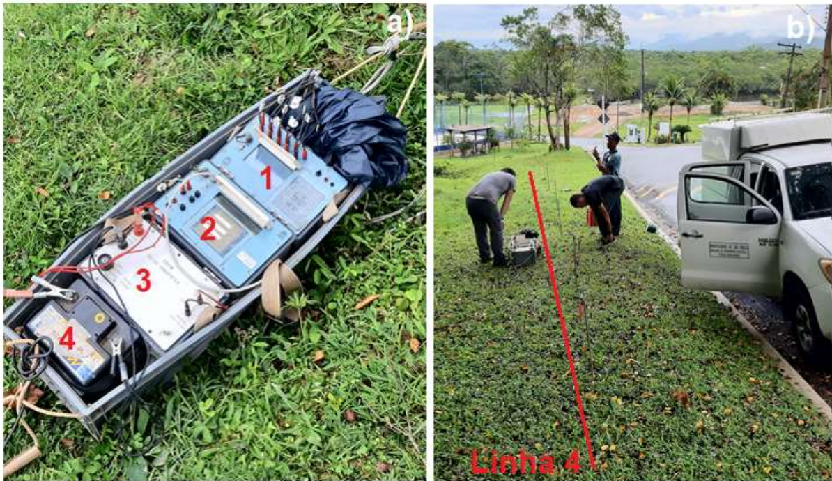
Figure 5 – a) Rho/IP system used in the electrical path, 1(receiver), 2(transmitter), 3(DC/DC converter), 4(battery). b) Data survey on Line 4. Source: Own authorship.
