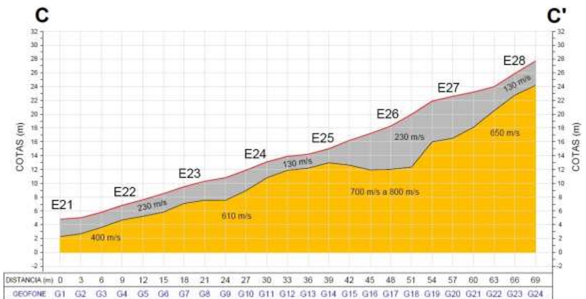
Figure 9 – Inferred seismic model for line 3, on the hillside. Source: Own authorship.
