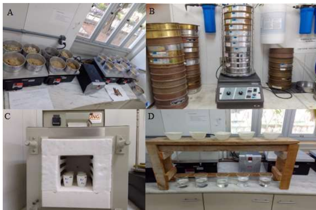
Figure 03 – Laboratory methodology. Samples in drying (A); Set of sieves on the ROT-UP device (B); Samples the muffle furnace (C); Washing of samples (D).
