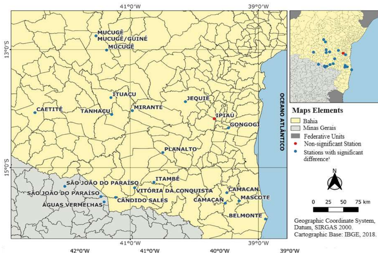
Figure 3 – Spatial distribution of the rainfall stations analyzed during the study, with a representation of the stations that showed and did not show a significant difference at the 5% significance level in the stationarity test of the data series.
