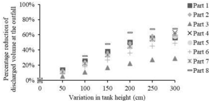
Figure 16 – Percentage reductions in volume discharged at the outfall.
