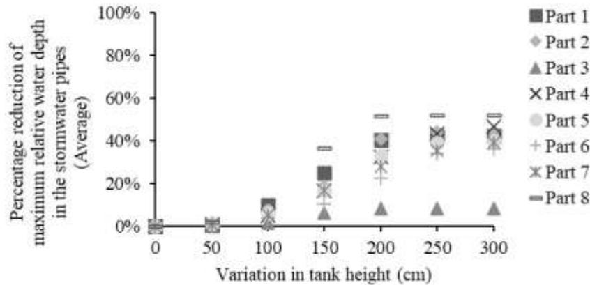
Figure 6 – Percentage reductions of maximum relative water depth in the stormwater pipes.
