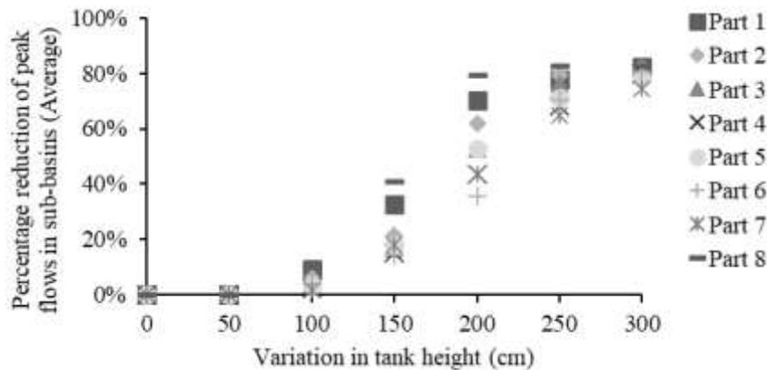
Figure 4 – Percentage reductions in peak flow in the sub-basins.
