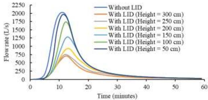
Figure 13 – Hydrographs at the outfall of Part 7.
