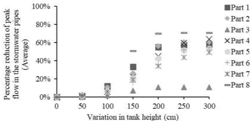
Figure 5 – Percentage reductions of peak flow in the stormwater pipes.
