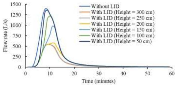
Figure 8 – Hydrographs at the outfall of Part 2.
