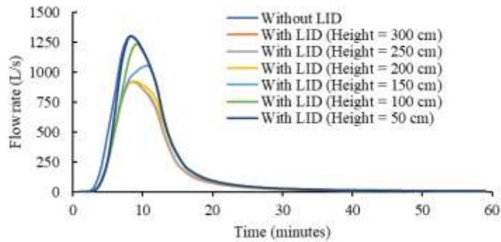
Figure 9 – Hydrographs at the outfall of Part 3.
