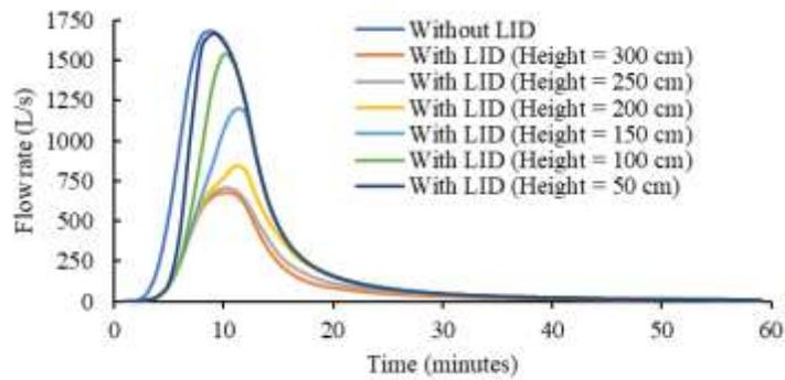
Figure 11 – Hydrographs at the outfall of Part 5.
