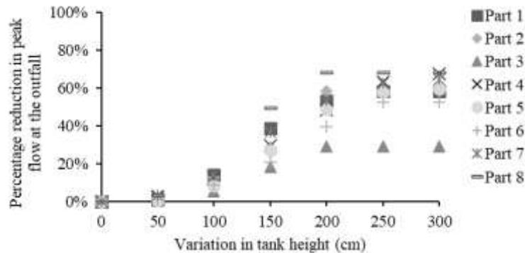
Figure 15 – Percentage reductions in peak flow at the outfall.
