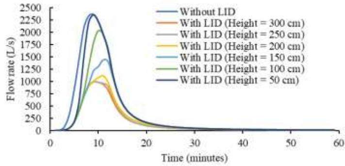
Figure 7 – Hydrographs at the outfall of Part 1.
