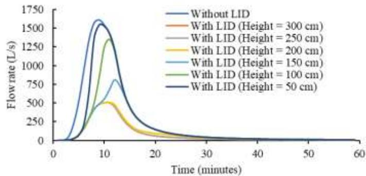
Figure 14 – Hydrographs at the outfall of Part 8.
