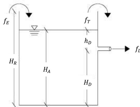
Figure 3 – Detention tanks simulation model in SWMM.
