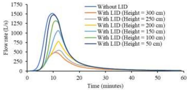
Figure 10 – Hydrographs at the outfall of Part 4.
