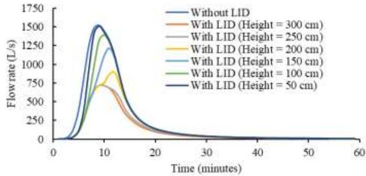
Figure 12 – Hydrographs at the outfall of Part 6.
