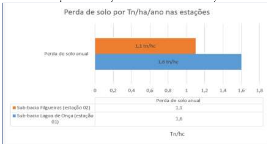
Graph 2 – Soil loss from the sub-basins under analysis
