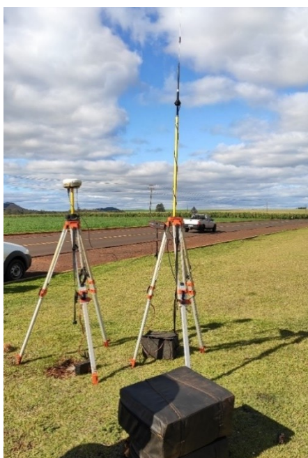
Figure 2 – Setting up the Trimble RTK R4 GNSS system.
