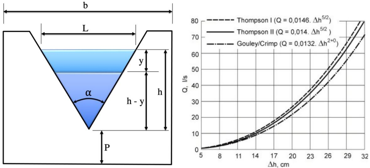
Figure 7 – Diagram of the Triangular Flow Meter.
