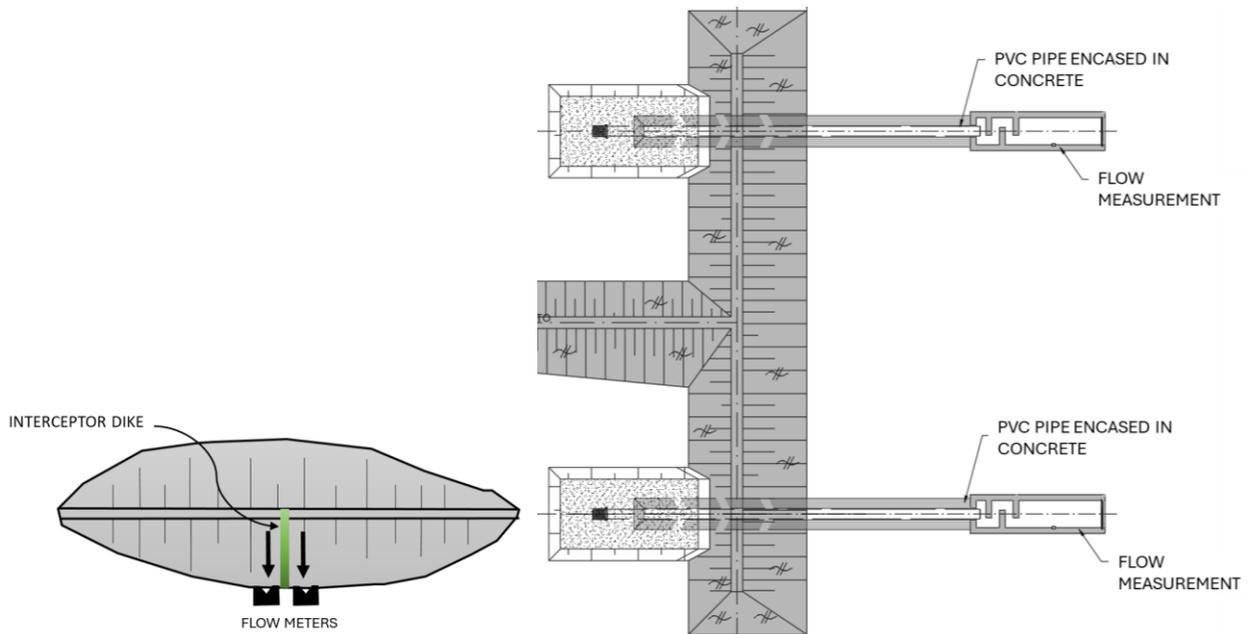
Figure 15 – Location of Flow Meter with Central Intercept Dike.
