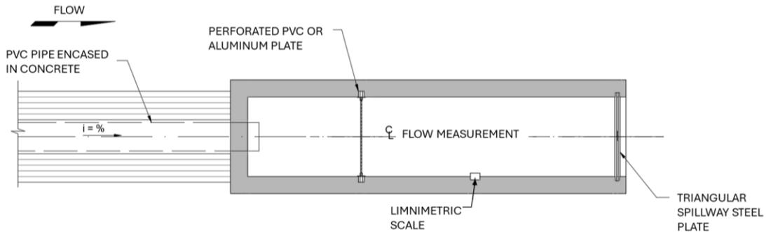
Figure 1 – Flow Measurement (Plan View).
