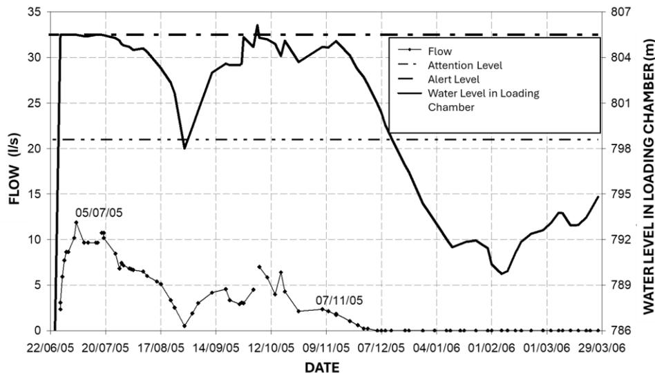
Figure 20 – Flow Meter of the Loading Chamber Dike at UHE Santa Clara.
