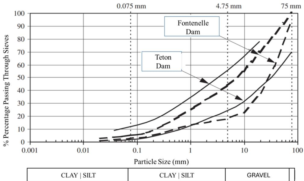
Figure 22 – Downstream Materials of Teton and Fontenelle Dams.
