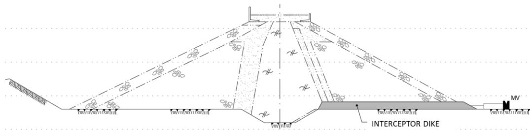
Figure 12 – Interceptor Dike in Earth Dam.
