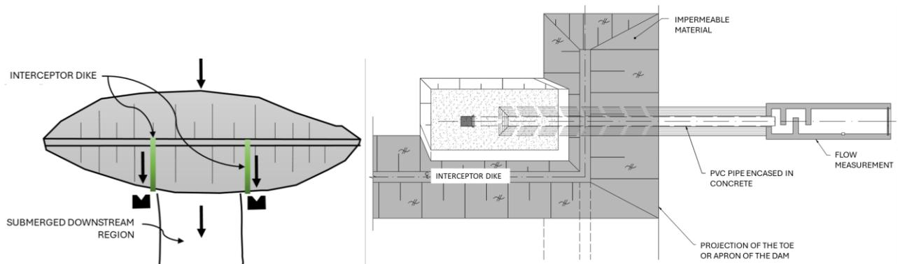
Figure 16 – Location of Flow Meters Limited to the Downstream Flooded Area.
