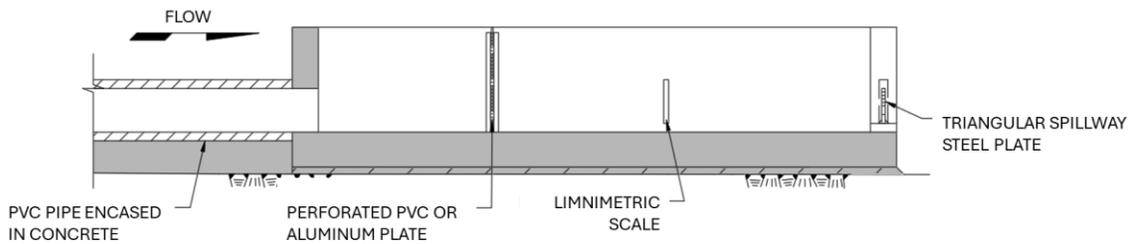
Figure 2 – Flow Measurement (Longitudinal Profile).
