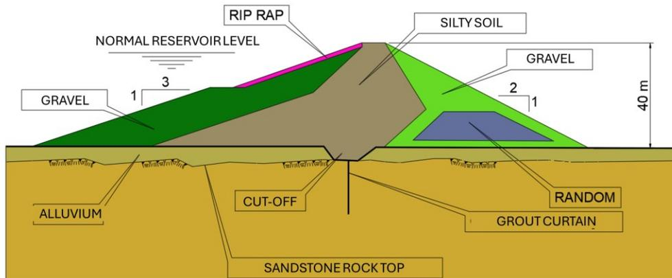
Figure 21 – Fontenelle Dam Section.
