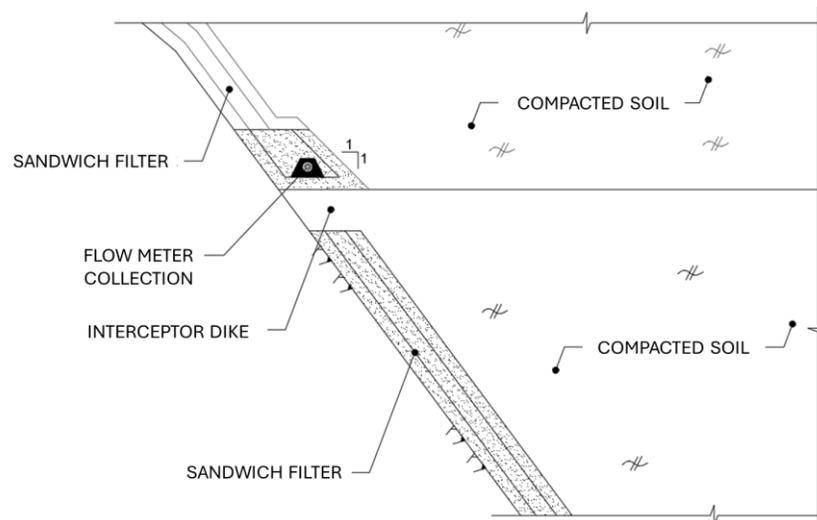
Figure 17 – Detail of the Interceptor Seal in Abutments.
