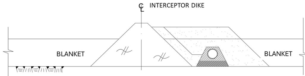
Figure 13 – Typical Detail of Interceptor Dike.
