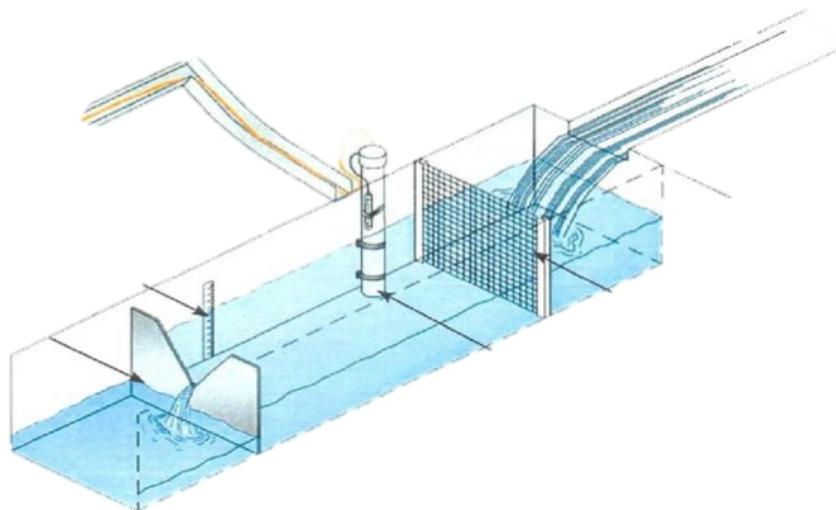
*Figure 10 – Diagram of the Triangular Flow Meter.
