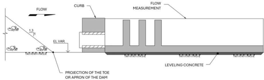
Figure 5 – Flow Meter with External Curb (Longitudinal Profile).
