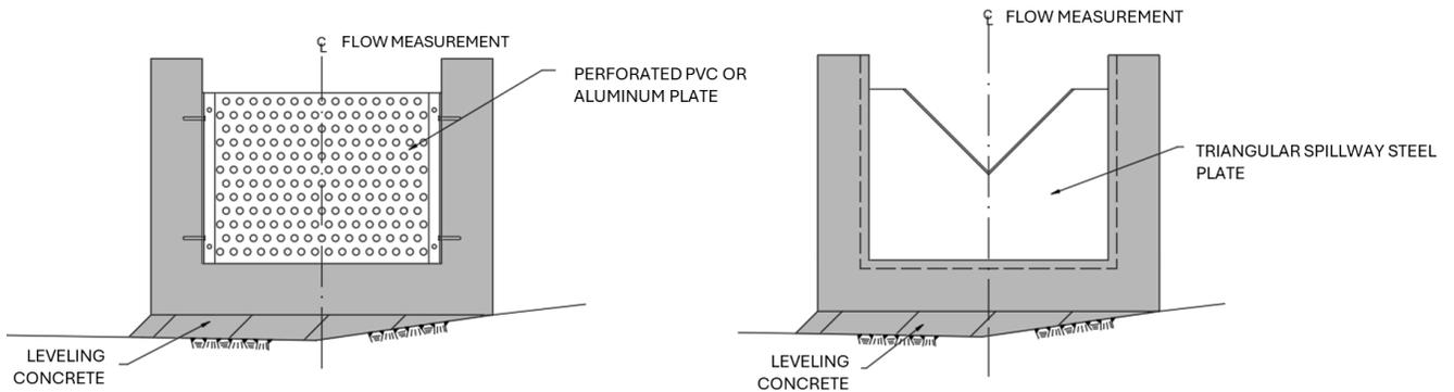
Figure 3 – Flow Measurement (Section and Elevation).
