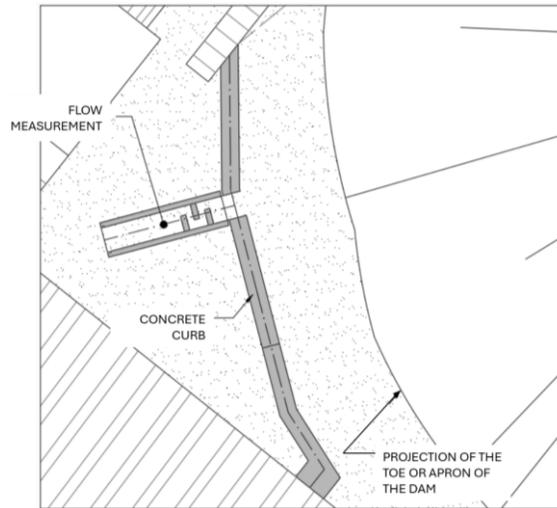
Figure 4 – Flow Meter with External Curb (Plan View).
