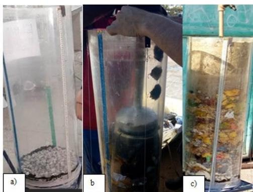
Figure 6 – Filling of lysimeters; a) Gravel b) USW compaction c) Soil compaction.
