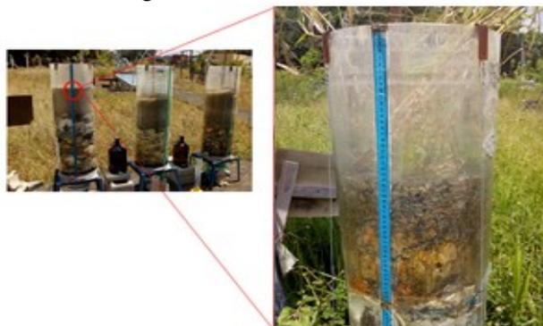
*Figure 8 – Manual measurement of settlements.
