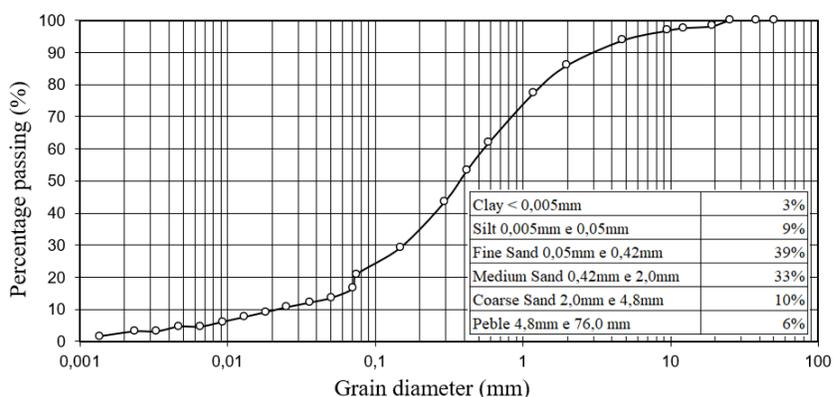
Figure 7 – Particle Size Distribution Curve.
