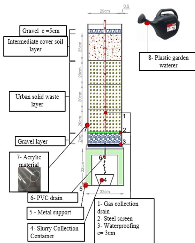
Figure 2 – Experimental lysimeter design.
