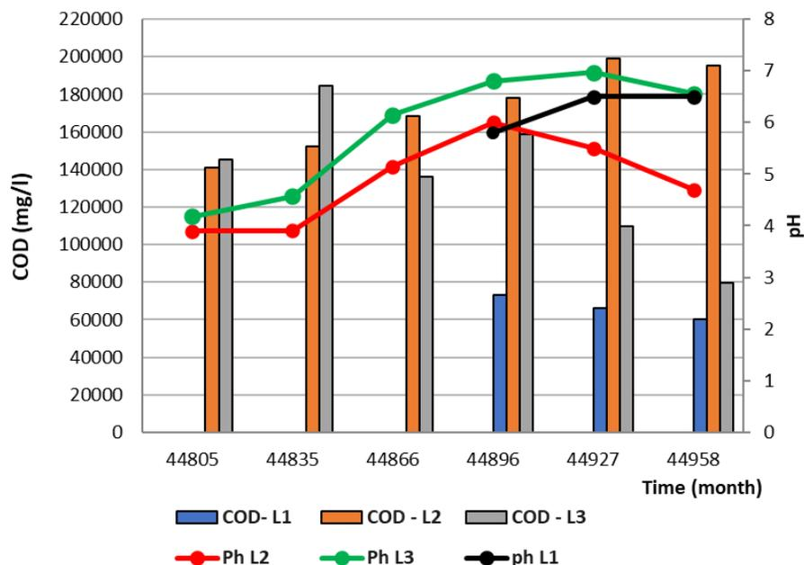
Figure 10 – COD and pH Lysimeter L1, L2, and L3.
