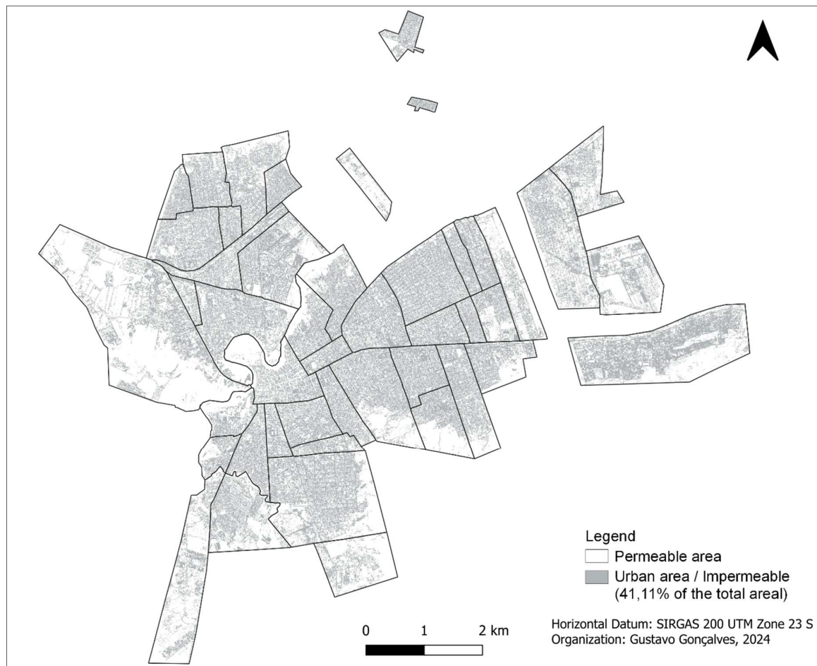
Figure 8 – Percentage of the total impermeable and non-permeable areas in the polygons of the neighborhoods of Barreiras, BA. Source: Authors (2024)
