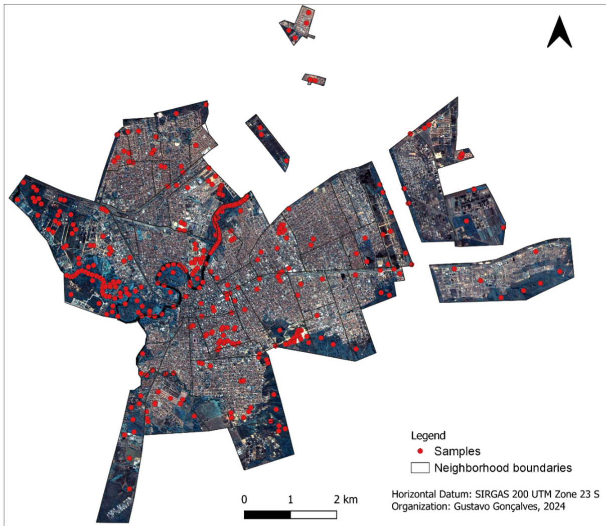
Figure 2 – CBERS-4A fused image highlighting the samples used to separate the impermeable areas. Source: Authors (2024).
