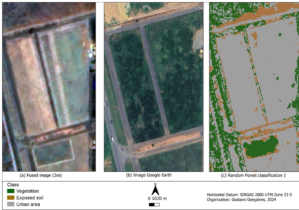
Figure 3 – Example of image classification illustrating the confusion of vegetation pixels with urban areas. Source: Authors (2024).
