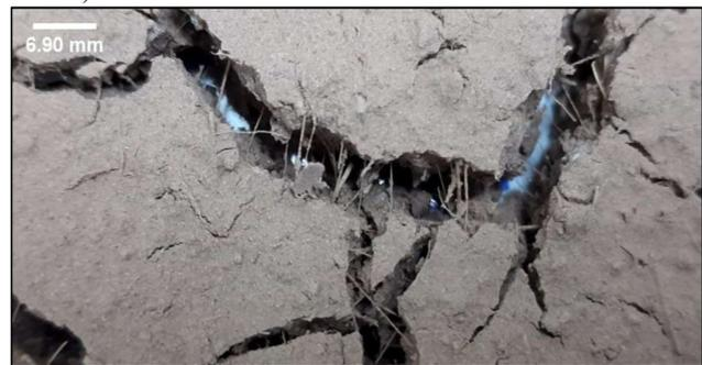
Figure 7 – Interaction Soil-fibers: a) after compaction for the soil+1% fiber mixture; b) In the Crack Formation Process. Source: Authors (2024).
