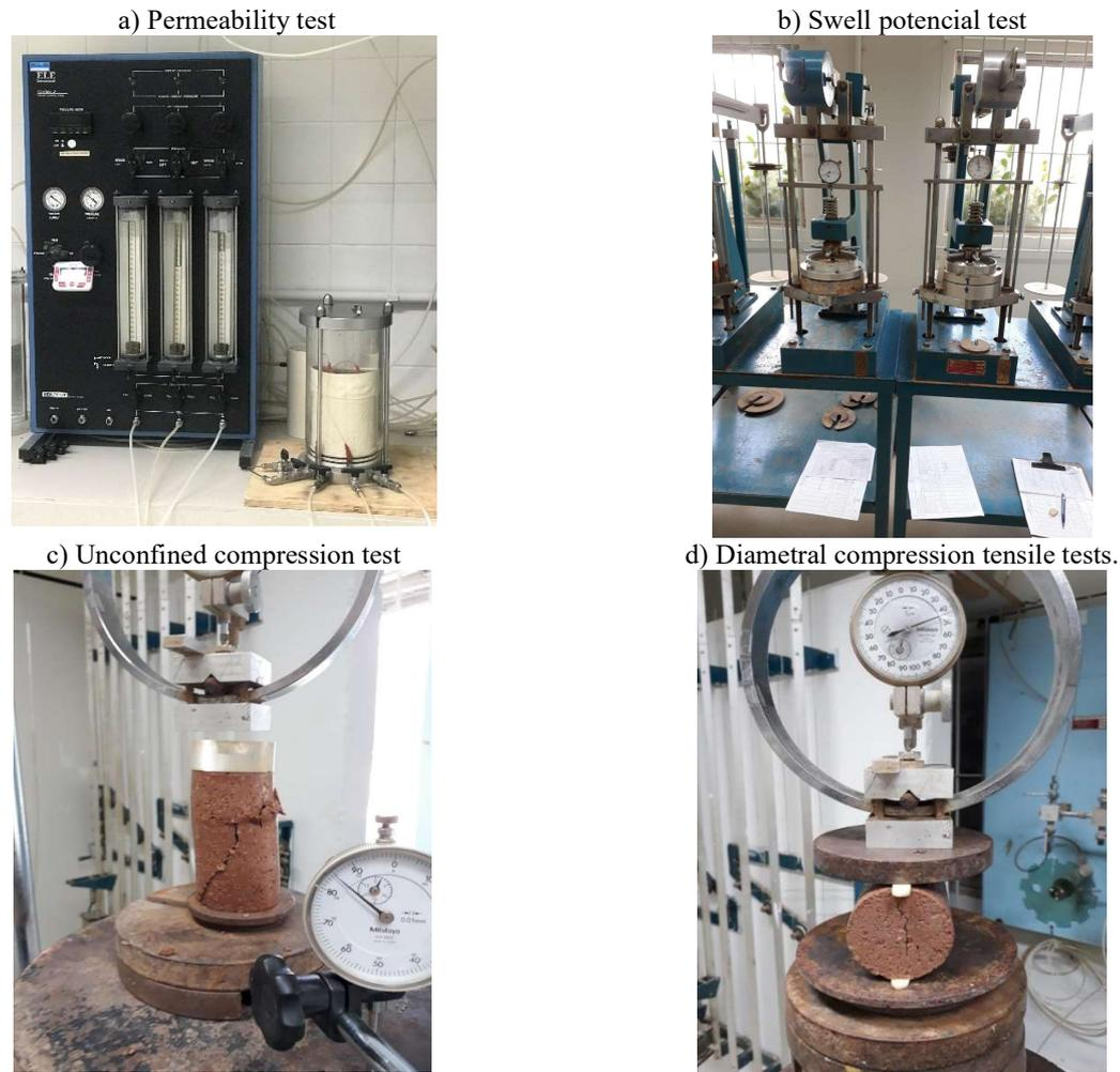
Figure 1 – Hydromechanical Tests: a) Permeability test ; b) Swell potential test; c) Unconfined compression test e d) Diametral compression tensile tests.
