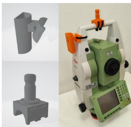
Figure 4 – Support brackets developed for reciprocal observations. Source: Authors (2024).
