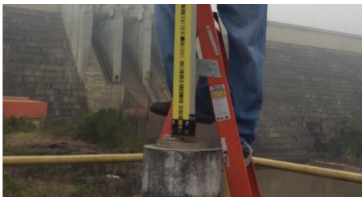
Figure 5 – Geometric leveling on the forced-centering pillar.
