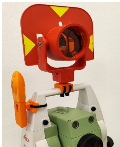
Figure 2 – Prism installation on the total station handle. Source: Authors (2024).
