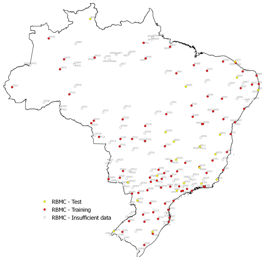
Figure 3 – RBMC stations randomly selected for training (80%) and testing (20%) the machine learning models. Source: Authors (2024).
