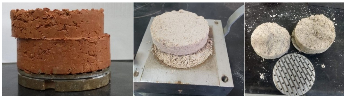
Figure 5 – Direct shear tests: images of the test specimens after shearing. Source: Authors (2024).
