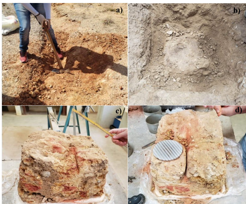
Figure 2 – Collection (a) and preparation of undeformed samples (b, c, d). Source: Authors (2024).
