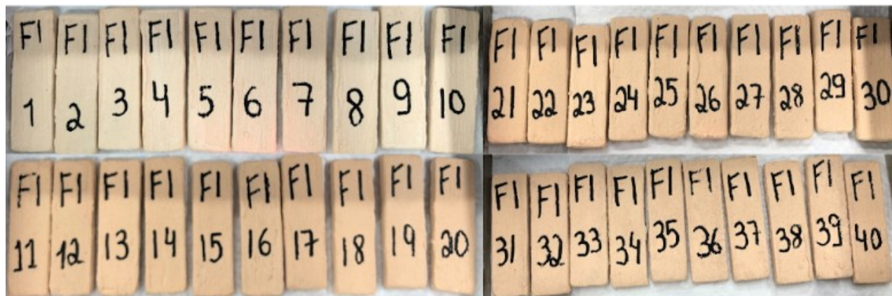
Figure 4 – Sintering of the glazed pieces at 1000°C – (F1).
