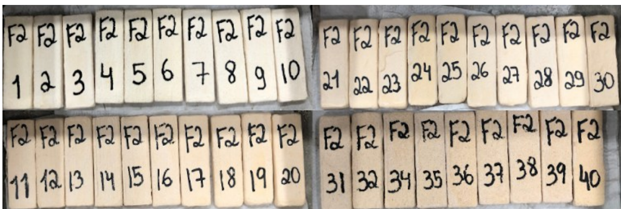
Figure 5 – Sintering of the glazed pieces at 1100°C – (F2).
