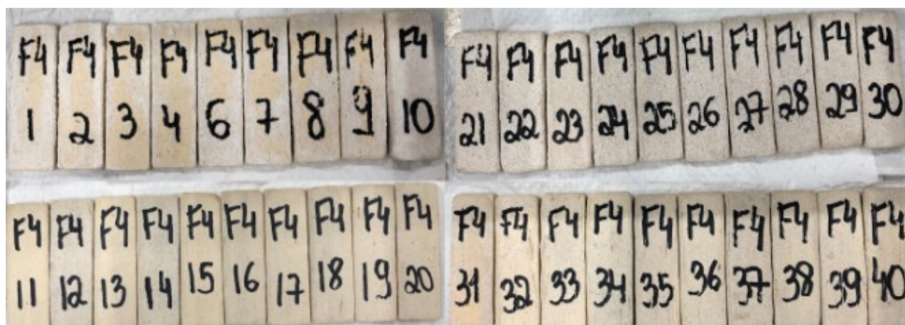
Figure 7 – Sintering of the glazed pieces at 1200°C – (F4).
