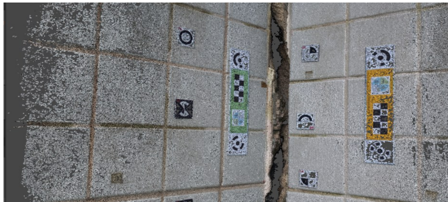
Figure 5 – Dense point cloud generated in Agisoft Metashape. Source: The authors (2026).
